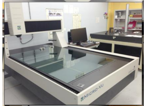
CNC– Vision & Touch Probe CMM, (MICRO-VU 1604 UC, 41” X 65” X 15.7”) (For The Larger Parts)
