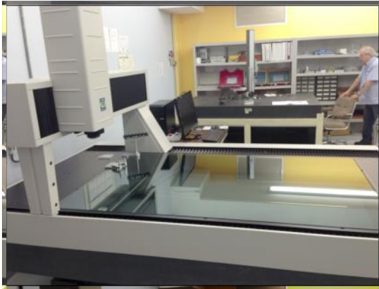
CNC– Vision & Touch Probe CMM, (MICRO-VU 1604 UC, 41” X 65” X 15.7”) (For The Larger Parts)
