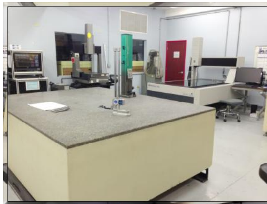
CNC– Vision & Touch Probe CMM, (MICRO-VU 1604 UC, 41” X 65” X 15.7”) (For The Larger Parts)
