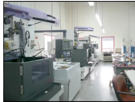
Wire EDM Multi-Axis ( X = 19.5", Y = 14.5", Z = 16" )
